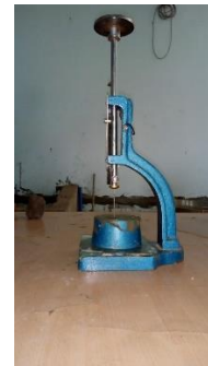
Figure 3.6 Initial and Final Setting Time Test
