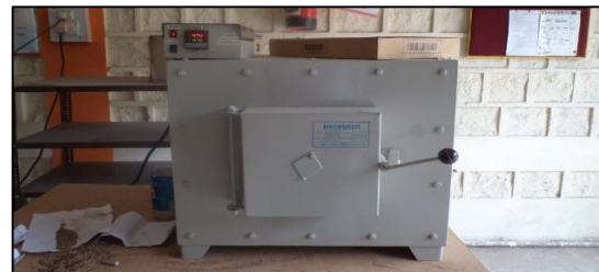
Figure 3.2 Bagasse burned in Muffle type Furnace
